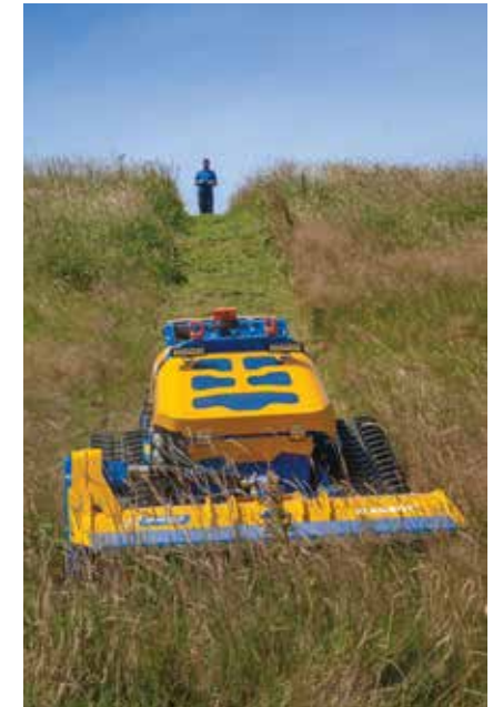
Working range All Flailbot models have an impressive working range of 150m (492').
