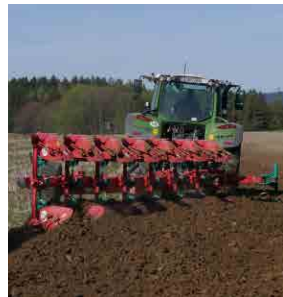
Packer arm and packers available for immediate re-consolidation
