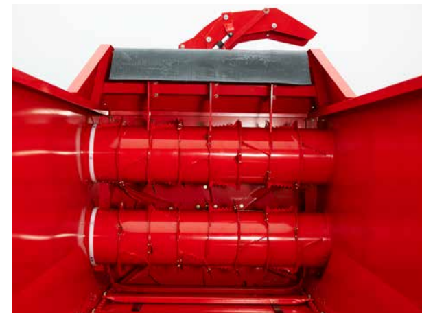
Two drum solution designed to handle large volumes of material.
