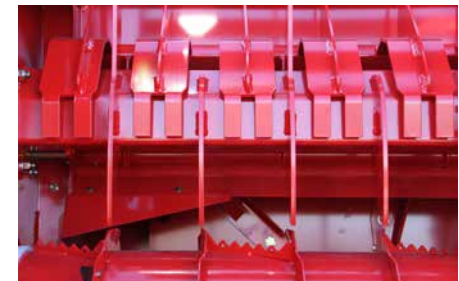
DFCS disengaged for maximum flow through the flywheel.
