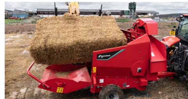
Generous access for loading of bale from the side.
