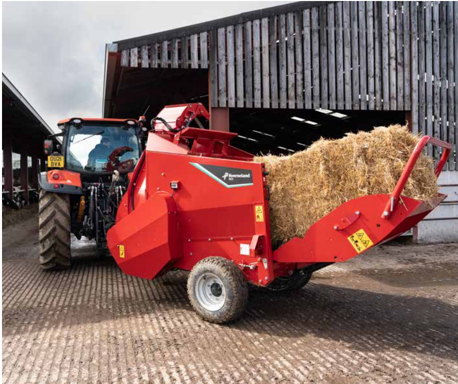
The extended drawbar ensures easier operation, especially when turning with larger tyred tractors.
