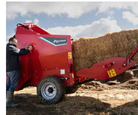
Operating both tailgate as well as floor chain in a safe distance from the moving parts by using the remote control placed on the side of the 860 series.
