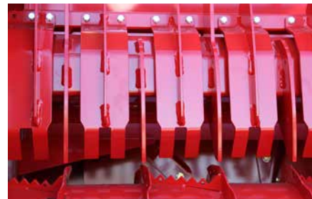
DFCS engaged to reduce the risk of blockages during loading and flywheel start up.
