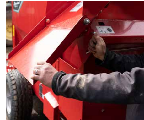
Adjustable slide for guiding material away from the wheel of the bale chopper.
