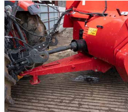
The extended drawbar ensures easier operation, especially when turning with larger tyred tractors.
