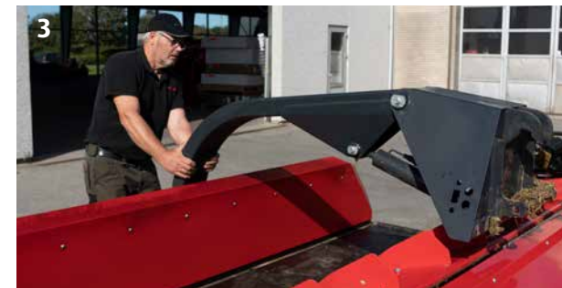
3 Lower the mowing units and the BX belt automatically comes off.
