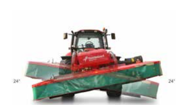
Vertical adaptation of 24° to adjust to uneven fields.
