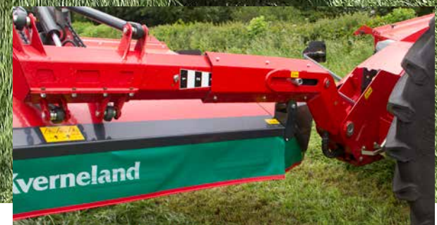
Overlap and effective working width is adjusted hydraulically on Vario models.
