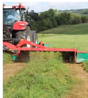
The large compensating spring ensures excellent flotation across the full mower width.
