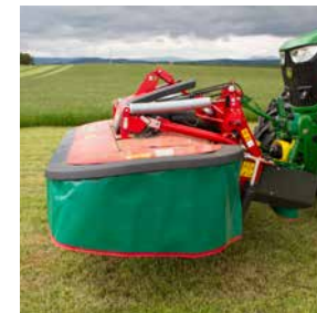
Generous ground clearance for headland turns of 420mm to pass large swaths without damaging them.
