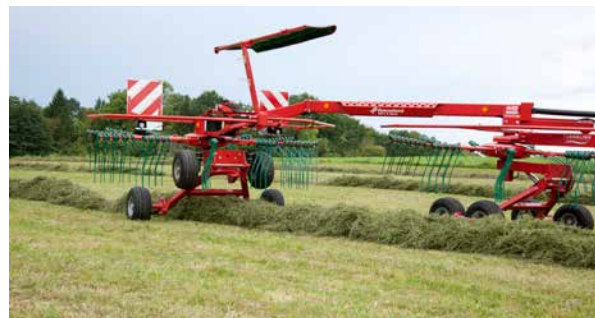
Turning on headlands: Kverneland is equipped with the QuickLift system as standard. This ensures a lifting height of 50cm to easily over cross existing swaths.
