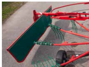
Automatic fold-able swath board with parking stand.
