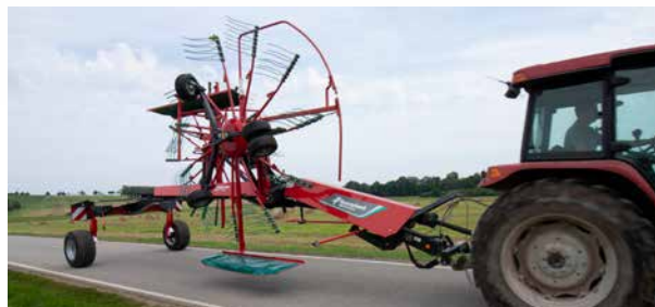
Transport height below 4m.
