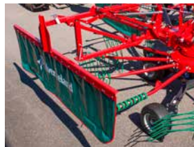
Automatic fold-able swath board with parking stand.
