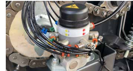
Automatic chain lubrication with individually adjustable outlets.
