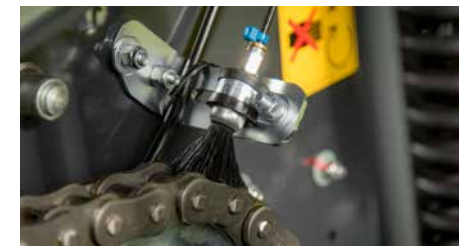
Automatic chain lubrication is standard on Kverneland 6500F.
