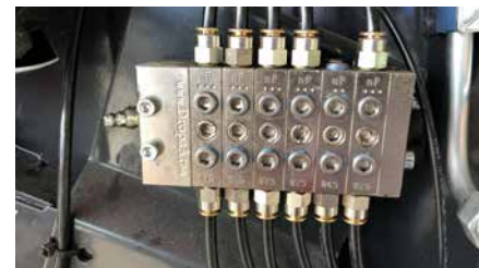
Remote grease bank for bale chamber roller bearings.
