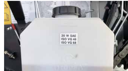
Large capacity chain lube tank.
