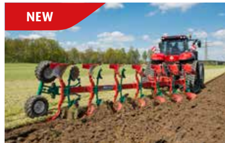
LO (On-Land) Easy switch In-Furrow/On-Land ploughing. Smooth turnover. Easy to lift and to pull. NEW: optional TTS for safer transport.
