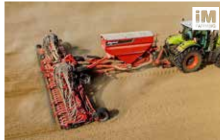
Pneumatic Seed Drill DG II DG II - the flagship for up to 140 ha per day! The “Active on” system for individual coulter pressure supports the easy handling and short set-up time! Equipped with the electric driven ELDOS metering system.
