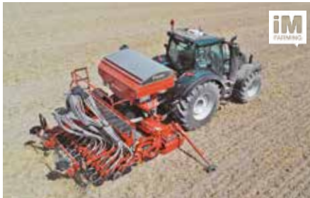
Pneumatic Seed Drill e-drill maxi plus Seeding and fertilising in one pass. The hopper capacity of max. 2,100 litres is divided into an adjustable ratio of 60:40, 70:30 or 100:0. With two independently working ELDOS either side.
