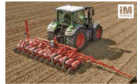
Monopill PH (6 m & 9 m) The convenient and time saving parallel hydraulic folding ensures a transport width of a maximum of 3.0 m.
