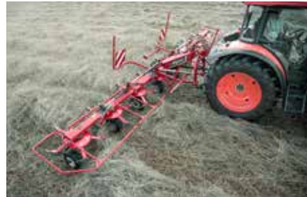
8460-8480 CompactLine Two compact models with 6 or 8 rotors and 6.05-8.05 m working widths. Standard fitted with oscillation dampers.
