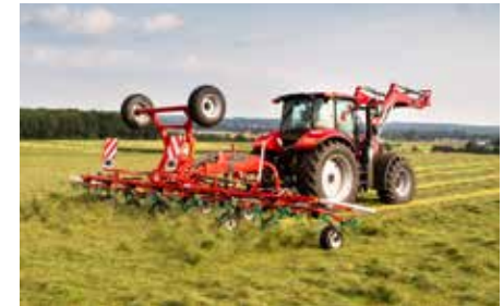
8590 C-85112 C ProLine The Kverneland 8590 C with 9 m and 8-rotors and the new 85112 C with 11.2 m and 10-rotors are carrier frame tedders.
