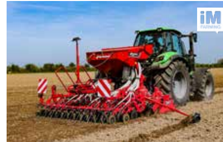
Pneumatic Seed Drill s-drill The s-drill is the heavy-duty version of the DA. It is a high-performance machine for larger farms and estates.
