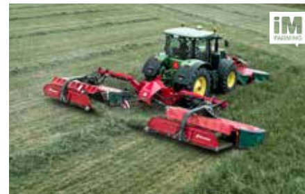
53100 MT Vario BX Series QuattroLink suspension, Vario overlap adjustment, optional detachable BX belt for maximum productivity.
