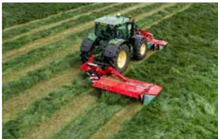
3200 MN/MR/MT Series Fitted with either rigid nylon tines, roller conditioner or SemiSwing steel tines, to suit various crops and conditioning demands.
