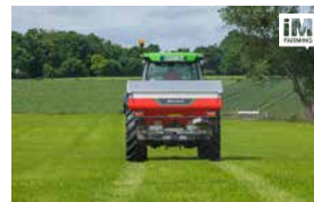
Exacta CL EW An ISOBUS compatible weighing spreader with speed related spreading and high frequency automatic calibration.
