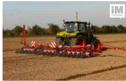
Unicorn PH (6 m & 9 m) Easy conversion from transport to working position. The transport width of all models is a maximum of 3.0 m.
