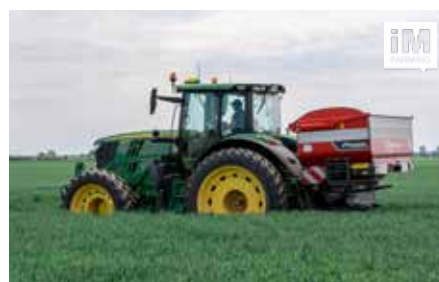
Exacta TL GEOSPREAD® iDC iDC means intelligent Disc Control. For more accuracy in border spreading in all conditions due to the independent disc speed left and right.
