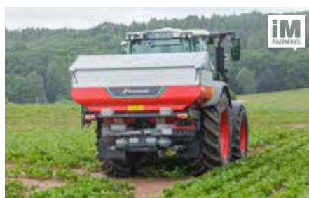
Exacta CL and TL GEOSPREAD® Unnecessary overlap is set to a minimum, because of section control. The total benefit of GEOSPREAD® combined with speed related spreading and GEOPOINT® headland management can be up to 15%.
