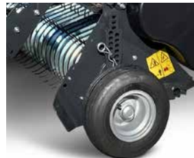
Large diameter easily adjustable guide wheels.
