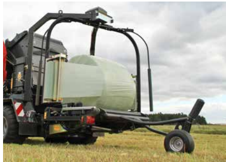
Twin satellite wrapper with 2 pre-stretchers and 4 endless belts for fast and stable wrapping.
