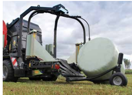
Bale turner option. During transport the kit is automatically pivoted into a safe position on the wrapping unit.
