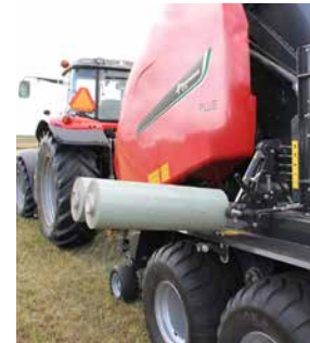
Twin cassettes for 10 spare film rolls operated hydraulically.
