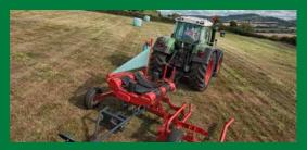
Turntable with two driven rollers designed for a high bale stability and smooth even rotation.
