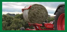
Hydraulically operated loading arm, and a low loading height, provides fast transfer of bale from arm to turntable.
