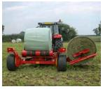
The short lifting height provides fast transfer of bale from arm to turntable.
