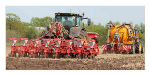
By using GEOCONTROL® there are no overlaps. Costs for fertiliser, seeds and chemicals are saved as well. GPS control of the tractor is advised for the Strip-Till. The implementation of the RTK signal (+/-2cm) guarantees high precision. The working width of the Stip-Till implement should correspond to the working width of the precision seed drill or have its double width at maximum.
