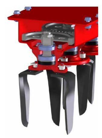
The Kverneland M series is a medium-sized power harrow for tractors up to 140HP. It is the lightest model in the Kverneland power harrow range but not only the heavy-duty headstock follows the design concept of the robust S series but also the self-supporting trough construction, as well as the optional 'Quick-Fit' tine holders and double conical bearings offer the optimum performance.
