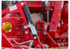
On the hydraulic foldable power harrows the working depth setting is adjusted by spacers at the cylinders. The working depth is changed hydraulically from cab. A parallelogram linkage ensures that the power harrow is always in a horizontal position to the roller. Therefore, the packer roller scraper bar position is basically a fixed height to the ground, independent from the working depth.
