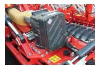
On the foldable Kverneland power harrows the main gear distributes the force to the sides. On each side is a gearbox separately overload protected which ensures a robust driveline up to 350HP. The rotor speed setting varies from 336 to 450rpm at 1000rpm PTO shaft. The F35 is equipped with a change gearbox.
