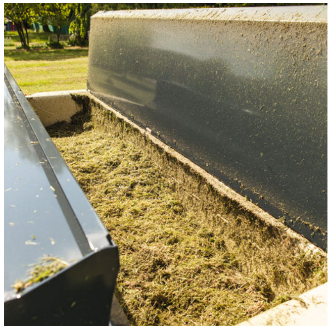
Compacted, cut material in the collection hopper
