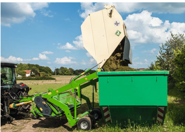
At up to 2.3 m high, the hopper can also be emptied into taller trailers or larger containers
