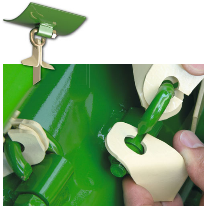
Tool-less conversion to scarifying – and done in seconds
