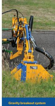
For protecting drive and machine during operation.
