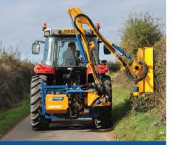
Hydraulic slew & breakout 110° of slew and hydraulic breakout makes the Osprey very adaptable.
