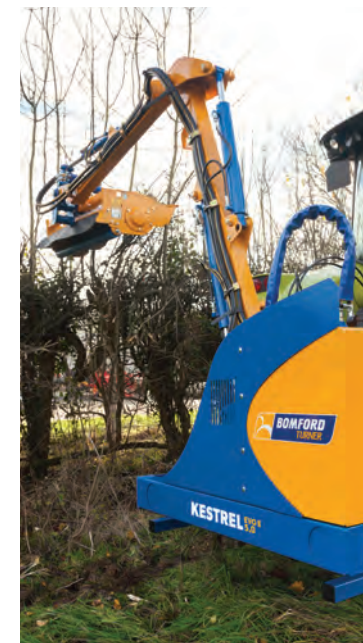
Parallel arm options Available for ease of operation when hedge cutting.
