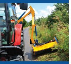
**Pro-Trim head** Fitted as standard with top drive motor.
