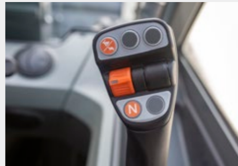
Comfortable joystick: Possible to switch between hare and tortoise on the joystick itself.
