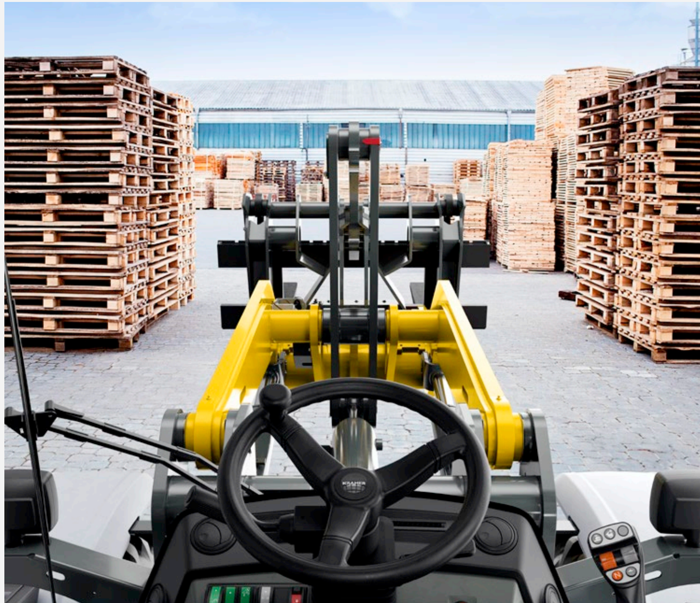
Excellent all-round visibility: a narrow cabin struts and panoramic glazing offer an optimal view on all sides.
