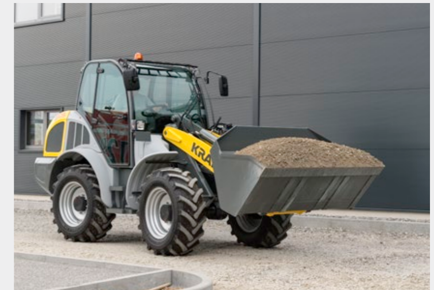
Front axle steering for increased stability during quick transport trips
