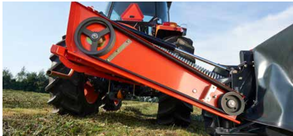
Four v-belts ensure excellent transfer of power.
