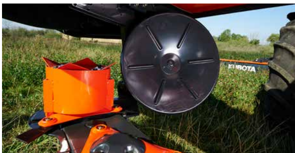
The machine is standard equipped with two swath discs, allowing a swath width of 2.2-2.4m.
