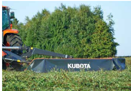
The centre suspended design enables fast and precise adaptation to ground contours.
