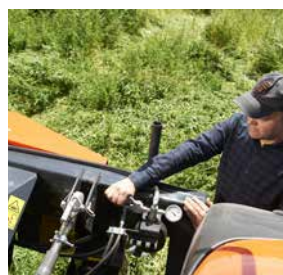
Hydraulic setting of ground pressure.
