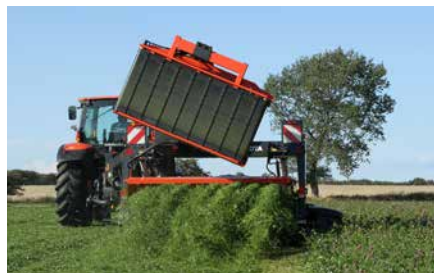
The crop is directed inwards, away from the unmovn crop.
