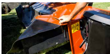
Integrated swath plates, easily adjusted to correct swath width.
