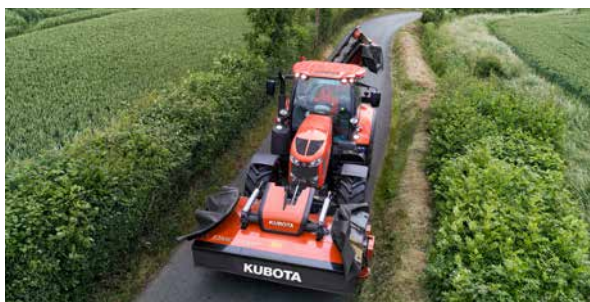
Hydraulic folding of FlexProtect guards (optional).
