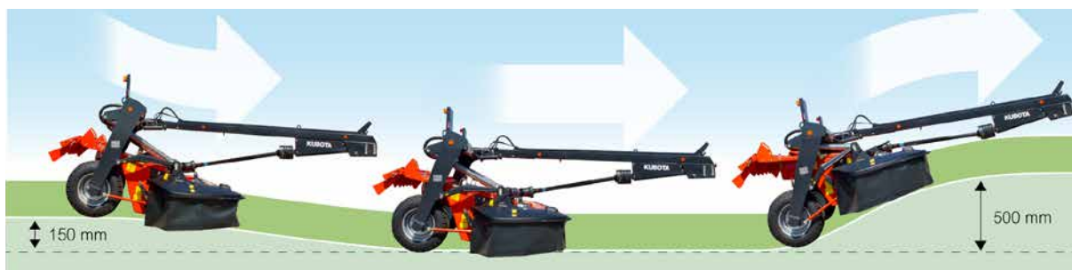
Easy adjustment of stubble height.
