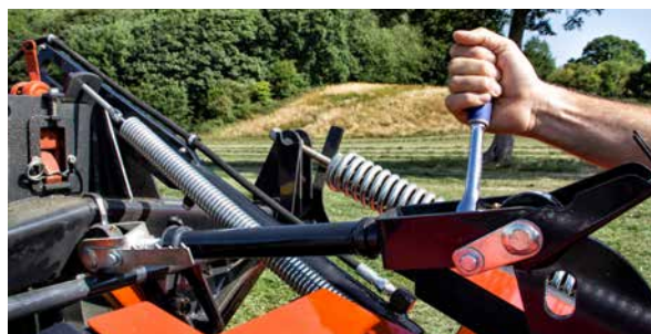
Stubble height adjustment is conveniently integrated directly into the suspension linkage. There is no need to tilt the A-frame of the tractor.
