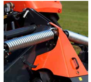
Large suspension springs, optionally with hydraulic setting of ground pressure.
