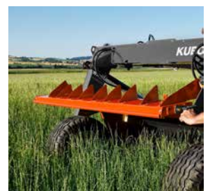
Dismount the two deflector doors and you are ready to mow.
