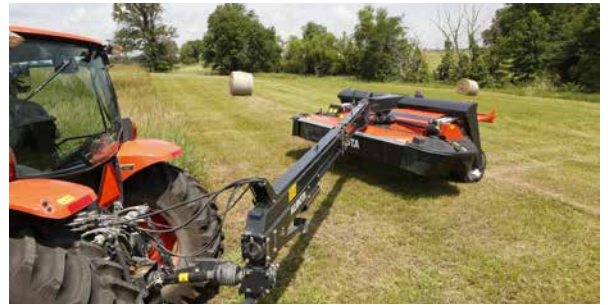
A lifting height of 500mm, ensures excellent ground clearance for transport and during headland turning.
