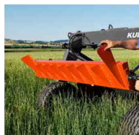
Changing from swathing to wide spreading is a one-man job. Simply turn the rear plate 180°.
