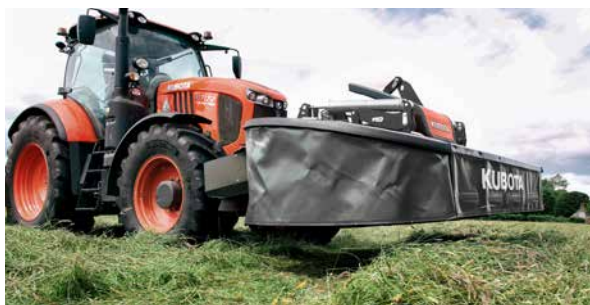
Generous ground clearance for headland turns of 420mm, to pass large swaths without damaging them.
