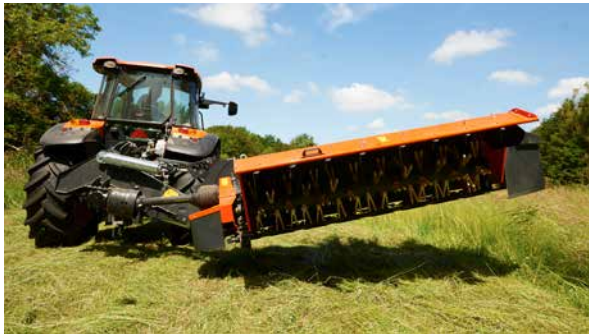
Lift on headland with ample clearance to existing swaths.
