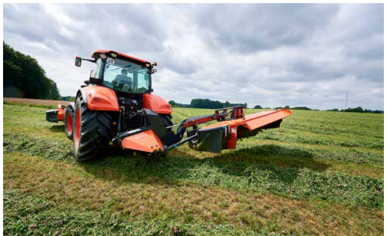
Minimum 500mm ground clearance across the complete mowing unit during headland turns. Mowing unit is raised and carrying arm tilted to a 10° angle.
