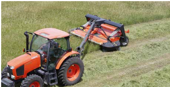
The mower can be operated on either side of the tractor...
