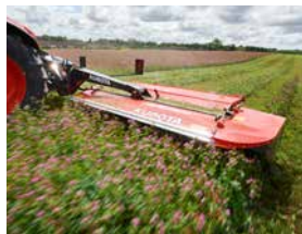
Centre suspension for even weight distribution across the entire working width.
