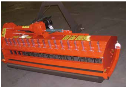
The Kubota SE3000 series can be equipped with rake tines to improve chopping on prunings.
