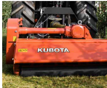
The SE1001 is equipped as standard with a rear roller which allows accurate control of cutting height.
