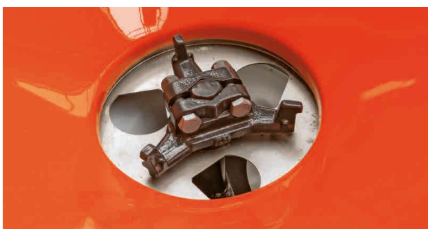
Agitator ensures even feed of the fertiliser
