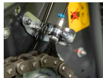
Automatic chain lubrication is standard on BF3500.
