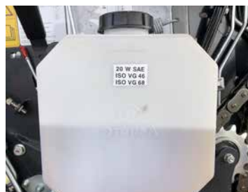
Large capacity chain lube tank.
