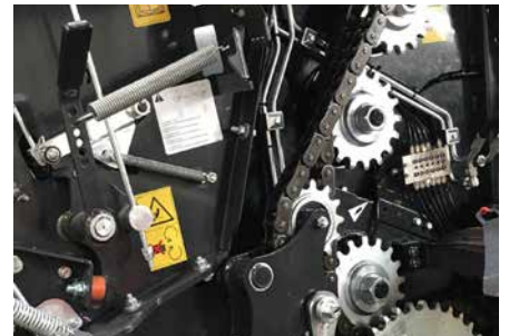
1¼” High specification ‘HBC’ chains are utilised on all bale chamber and rotor drives.
