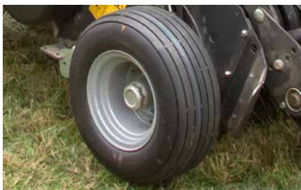
Generous flotation tyres with simple height adjustment.
