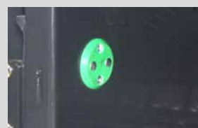
Moisture sensors located inside bale chamber.
