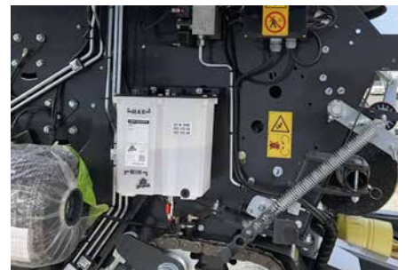
Rigid steel pipes for hydraulic circuits.
