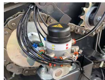
Automatic chain lubrication with individually adjustable outlets.
