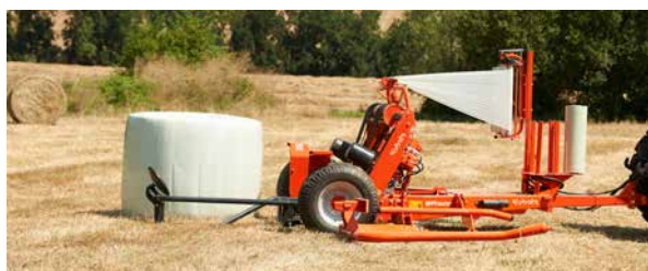
Fast and gentle on-the-move unloading with no need for a fall damper.
