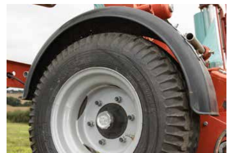
Mud guards reduce mud and dirt building up on the pre-stretcher and film rolls when operating in soft ground field and during transport.
