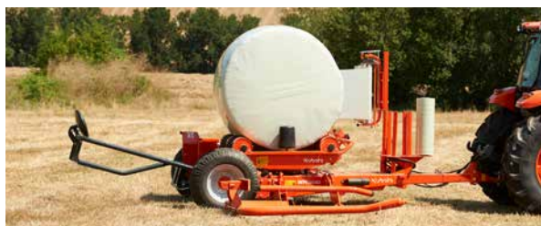
The adjustable loading arm with rear end stopper and inner support tube, allows the bale to be picked up and loaded on the move.
