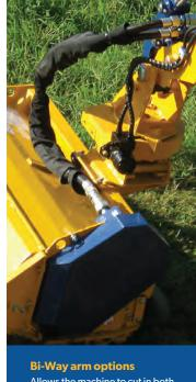
Allows the machine to cut in both forward and reverse directions.
