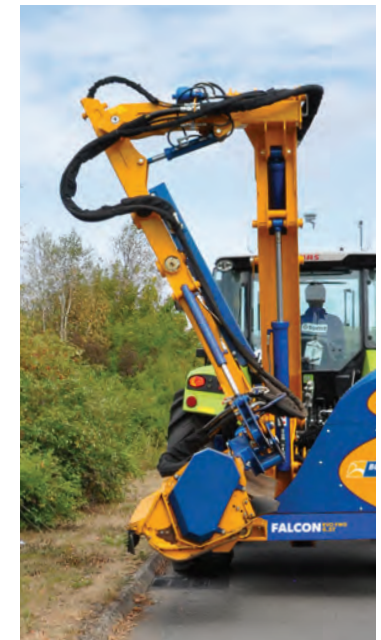
Transport bracket Supplied as standard for fast travelling on the road.
