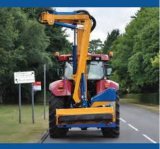
**Transport position** Folding 3rd arm allows compact transport position.
