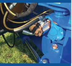
**Powerful 74hp hydraulics** For continuous use. Twin pumps with separate oil tank.
