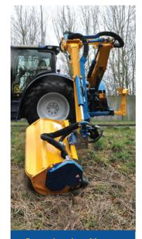
Forward reach position Enables mid-mounted head position with simplicity of rear mounted arm.
