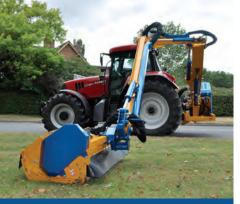
Impressive reach 3 arm design gives versatile reach characteristics for flexibility around obstacles.
