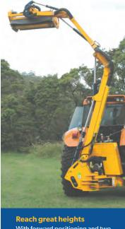
With forward positioning and two reach options of 7.1m and 8.0m.
