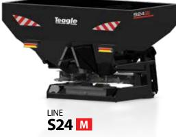
1,500 - 2,000 litre capacity 10-18 or 10-24 metre bout width Hydraulic Shutter Control
