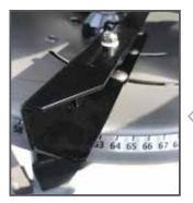
MT-vanes can be accurately adjusted in length and orientation from 18 to 36 metres according to the type of fertiliser, seeds and snail/ slug pellets. The operator, thanks to the clearly visible graduations, can adjust quickly without the need for tools.
