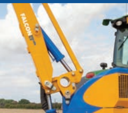
Parallel linkage Comes as standard to assist operator control.
