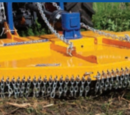
Protection Heavy duty chain guard protection.
