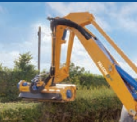
Forward reach position Enables mid-mounted head position with simplicity of rear mounted arm.
