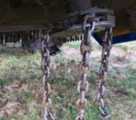
3 Heavy duty cutting chains 3 Chains per rotor in Grade 80 steel to work in stony conditions.
