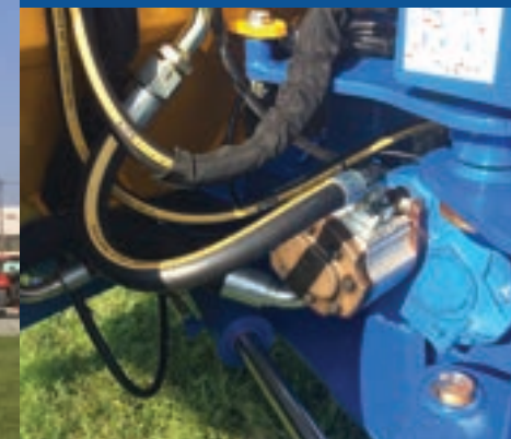
Powerful 74hp hydraulics For continuous use. Twin pumps with separate oil tank.
