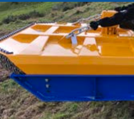
Adjustable skid height From 50 – 100mm.
