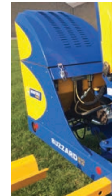
Fully enclosed hydraulics Keeping components protected from the elements.
