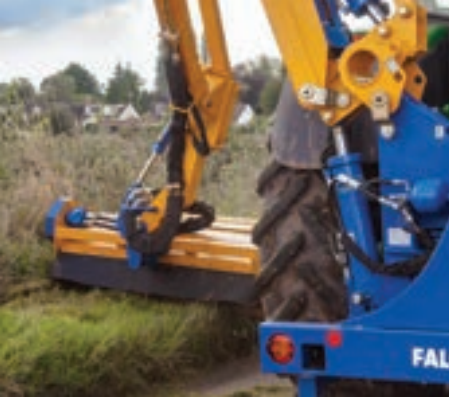
Arm float cylinder To aid grass cutting on roadsides.
