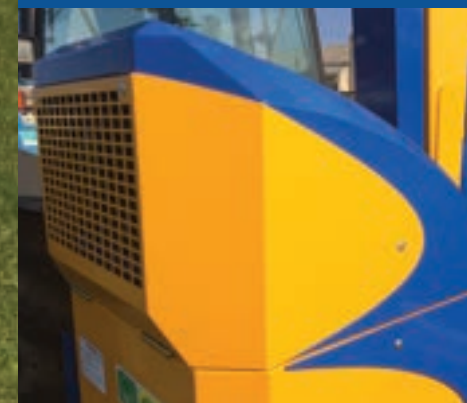
Oil cooler Standard on all models (cable controls as an option).
