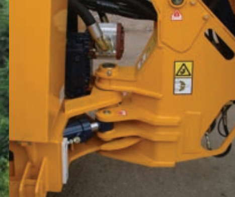
Heavy duty twin ram slew system Includes hydraulic breakout to protect machine operator.
